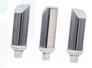
Heathfield LED G24 lamps are designed to replace the traditional compact fluorescent type. This 7w version offers in excess of 700lm. The unique design of the lamp offers a high light output that spreads light evenly giving a uniformed appearance. This product has been designed to give stable operation and low lumen depreciation.
