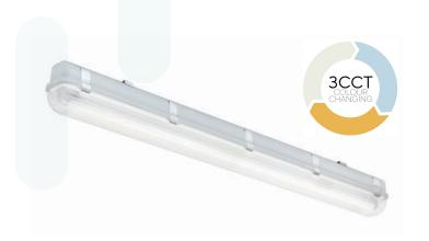
Heathfield LED Anti Corrosive fittings are designed to replace the traditional Anti corrosive fluorescent type. This 80w version offers in excess of 8,000lm. This range also offers an emergency version, dimming and sensor options are also available on request. This product also benefits from a colour changing switch enabling switching between 3000k, 4000k and 6000k.
