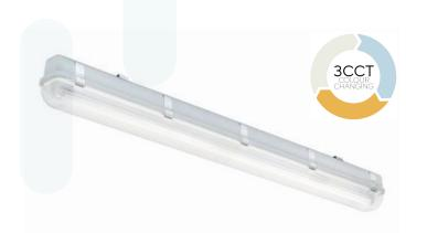
Heathfield LED Anti Corrosive fittings are designed to replace the traditional Anti corrosive fluorescent type. This 48w version offers in excess of 4,000lm. This range also offers an emergency version, dimming and sensor options are also available on request. This product also benefits from a colour changing switch enabling switching between 3000k, 4000k and 6000k.
